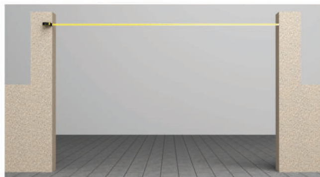
5 Mesurer en haut. Retenir la plus petite mesure; Consider the smallest distance between pillars (bottom, middle, top);
